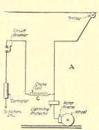
Fig. 154.—Protector on car—most desirable arrangement.
